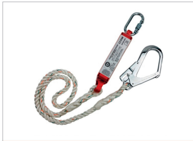
FBO-TE6102 Energy absorber lanyards Rope:1.3-2m Bearing:2.2 tons Energy absorber lanyards: 0.75m
